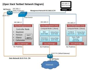
Figure 3. OpenStack Cloud Testbed
