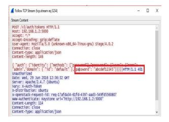
**Figure 4**. The API data exposed in plaintext during eavesdropping
